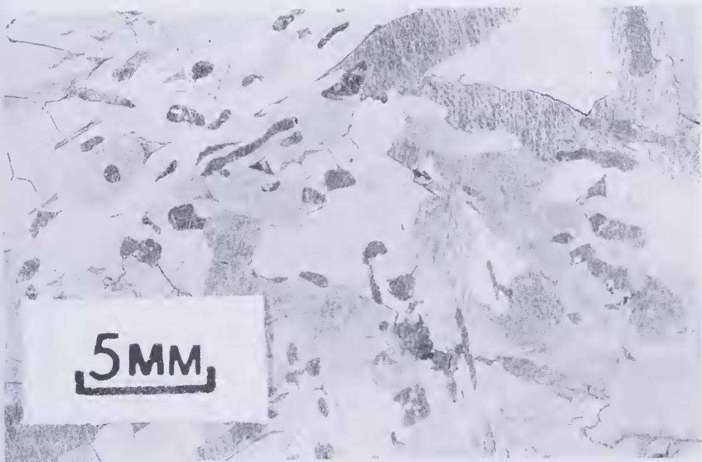
Figure 3.—A polished and etched section of the new specimen of the Youndegin meteorite shower.
